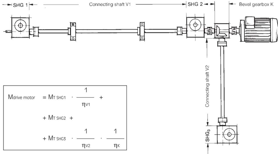
$$M_{\text{drive motor}} = M_{T \text{ SHG1}} \cdot \frac{1}{\eta_{V1}} + M_{T \text{ SHG2}} + M_{T \text{ SHG3}} \cdot \frac{1}{\eta_{V2}} \cdot \frac{1}{\eta_K}$$
