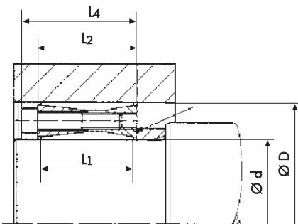
**Important:** Step in shaft or hub necessary for removal.
