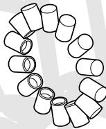
The elastic buffers absorb shocks and torsional vibrations, are resistant to oil and largely insensitive to temperature.
