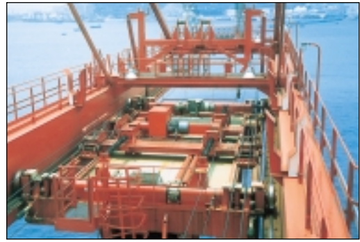
Anti Sway Mechanism, Ship to Shore Crane, Hong Kong. OEM: Morris Mechanical Handling.
