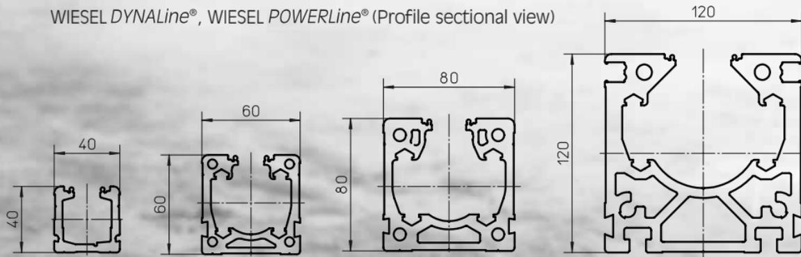
Tolerances of outer dimensions according to DIN 17615 part 3
